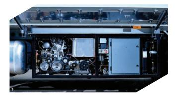
By using the liquid nitrogen engine as a secondary engine in trucks for cooling (instead of a second diesel engine), diesel consumption could be cut by up to 25%. The Dearman engine is also zero-emission and the company says it could one day be used in mass-market vehicles and for back-up cooling and power systems in buildings.
